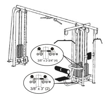
Figure 13. Mount the benches to the frame.
